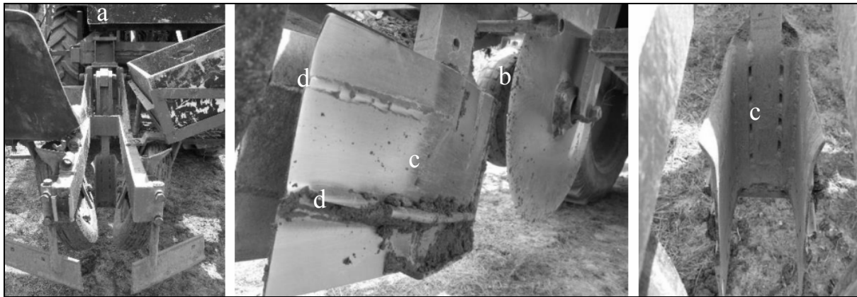
Fig. 1: The transplanter (a) is carried out on the three point hitch of a tractor. A transplanter is equipped with a disc coultter (b) mounted in front of the shoe (c) that is equipped with ribs (d) preventing compaction of furrow walls.
