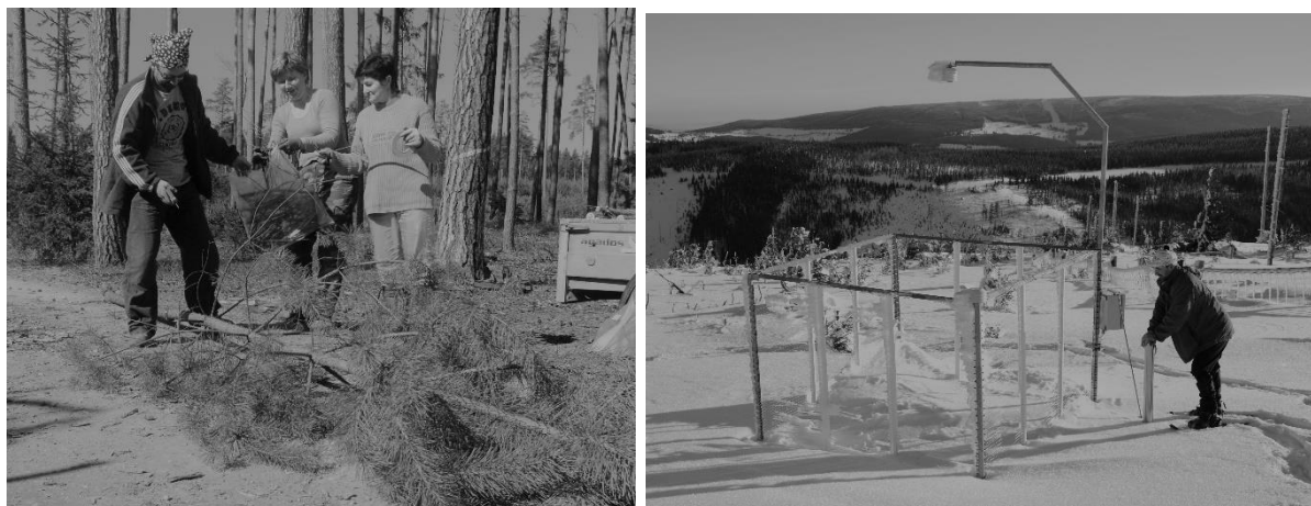
Fig. 3: Sampling of biomass components after experimental thinning in pine stand (left, 2014) and Snow Measurement System LDSMS2014 for continual measuring of snow water equivalent and snow depth (right, 2018).
